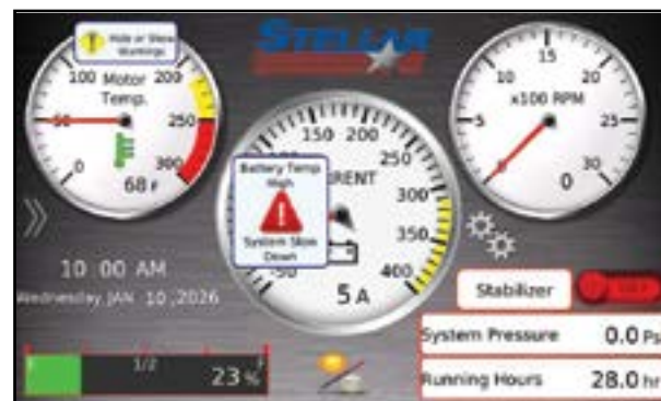
Figure 34: Faults. Battery Temp High.
