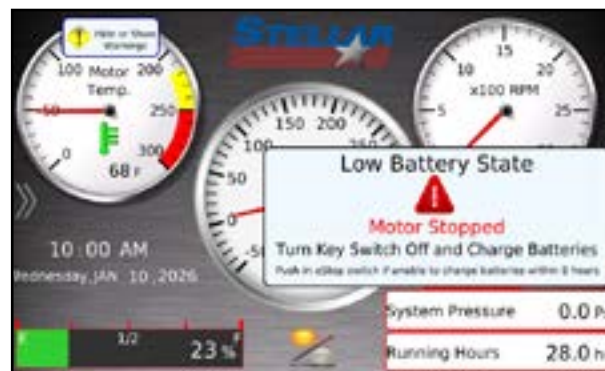
Figure 36: Faults. Low Battery State
