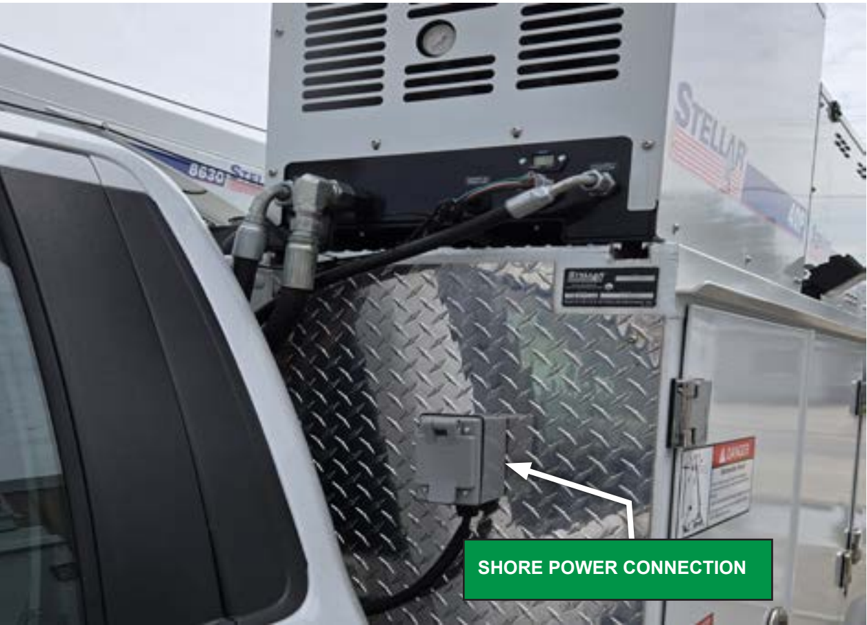
Figure 25: Charging, Shore Power
