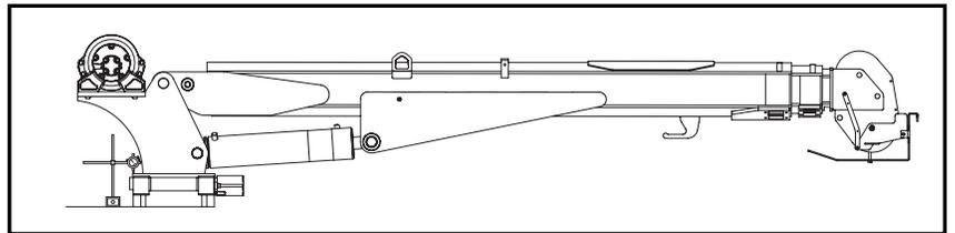
Step 6: Return the crane to vertical position. The dial indicator should return to calibration.
