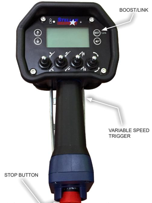
The radio remote allows for simultaneous functions. With practice, it is possible to use more than one toggle at the same time (Extension Out/Winch Down for example). See the Radio Remote Control Functions and Features pages later in this chapter for more information.
