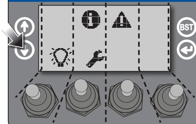
The third Shift Function Screen gives you access to diagnostic and information screens that can assist in crane trouble shooting and maintenance. Make a selection within 10 seconds or the screen will timeout and return to Crane Operating Mode. (See page 18 for more information.)
