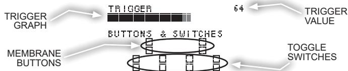
Button and switches can be tested by pressing or toggling. If the corresponding box does not light, there is a button (switch) or wiring malfunction.
