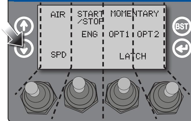
The first Shift Function Screen lets you activate several secondary functions remotely to increase productivity. Activate or deactivate optional function(s) within 10 seconds or the screen will timeout and return to Crane Operating Mode. (See page 16 for more information.)
