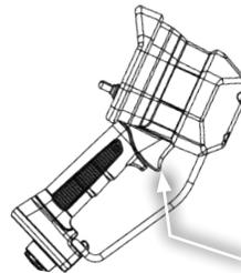
WHILE UNLINKED, DOUBLE CLICK THE VARIABLE SPEED TRIGGER AND THE SCREEN WILL SHOW CRANE MODEL AND CONTROLLER PROGRAM INFORMATION.
