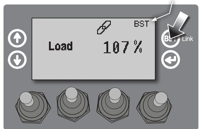
When the crane reaches 100% capacity, an overload shutdown will be initiated. The operator will need to set the load down and reposition the truck or activate the Stellar CDTpro Boost Mode.
