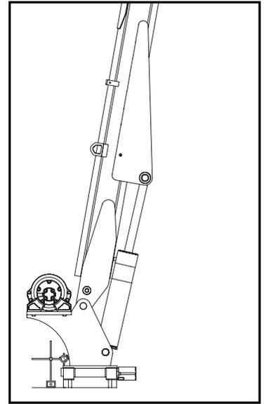
Step 4: Lower the crane to the horizontal position.
