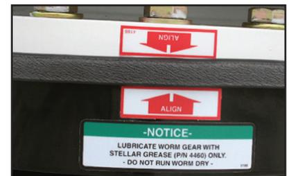
Note: Use alignment arrows located on the crane base to properly align the boom with the boom rest.
