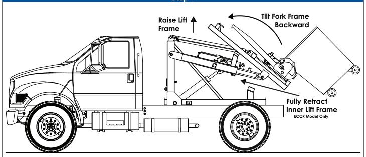
7. Raise the lift frame high enough to clear the truck frame. Fully retract the inner lift frame (ECCR Model Only). Tilt the fork frame all the way up so full contact is made with the rest pads.
