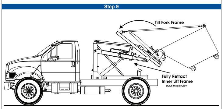
9. Tilt the fork frame all the way up so full contact is made with the rest pads. Fully retract the inner lift frame (ECCR Model Only).
