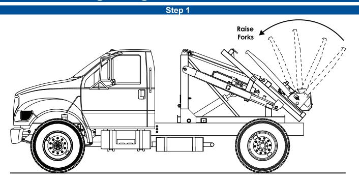
1. If the forks are in the extended position, manually rotate them to the stored position. Lock the forks into place with the fork stop pins.
