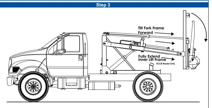
3. Tilt the fork frame forward and fully extend the inner lift frame (ECCR Model Only).
