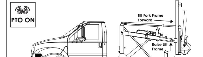
2. Engage the PTO and raise the lift frame high enough to clear the truck frame. Tilt the fork frame forward.
