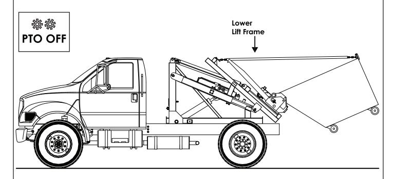
10. Lower the lift frame completely and disengage the PTO. Note: Check local DOT lighting regulations before transporting.
