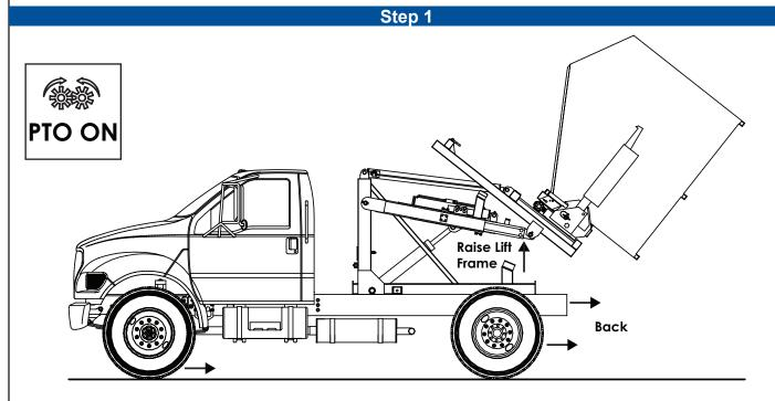
1. Back the truck up close to where the container will be placed. Engage the PTO and raise the lift frame high enough to clear the truck frame before tilting the fork frame.
