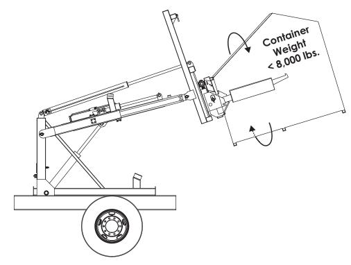
**AWARNING** Failure to tilt forks up before rotating container may result in container sliding off of forks with possible damage to equipment and injury to personnel
