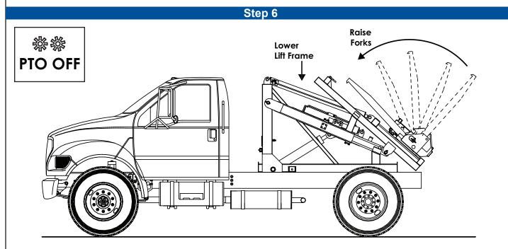
6. Lower the lift frame completely and disengage the PTO. Raise forks and lock in upright position.
