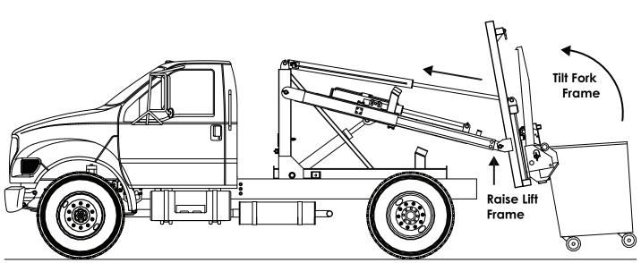
6. Raise the lift frame until the trunnion bars are securely located in the slots. Tilt the fork frame up until the container contacts the rubber bumpers. Put both trunnion bar stops in the 'locked' position (See next page).
