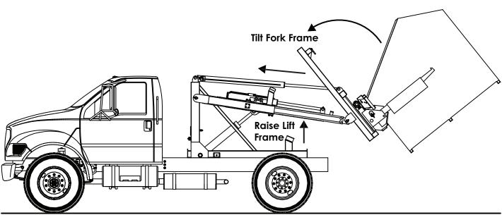
5. Raise the lift frame and tilt the forks up high enough to clear the truck frame.
