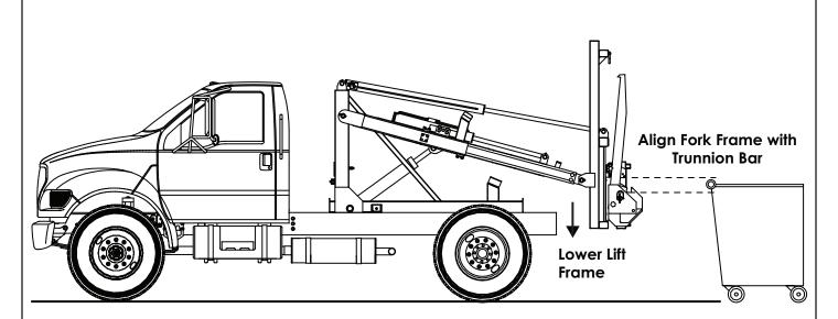
4. Align the fork frame with the trunnion bar on the container by lowering the lift frame and tilting the fork frame..
