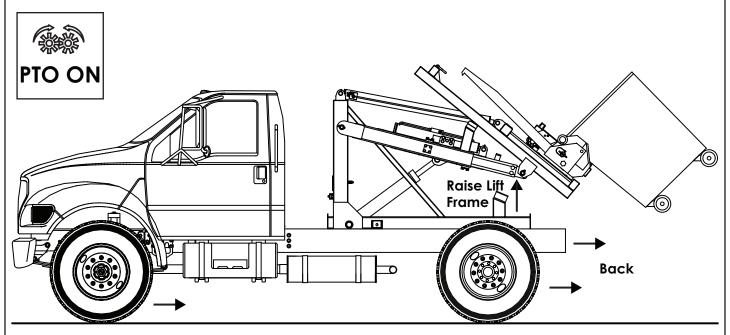
1. Back the truck up close to where the container will be placed. Engage the PTO and raise the lift frame high enough to clear the truck frame.
