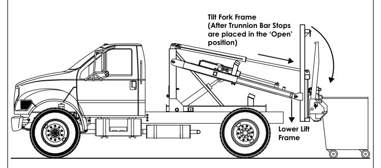
3. Lower the lift frame until the container is fully rested on the ground. Set the trunnion bar stops to the open position. Tilt the fork frame down enough to clear the trunnion bar slots.
