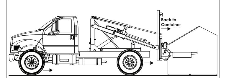
4. Slowly back the truck up to the container. Continue backing until the forks extend through the pockets and the container contacts the bumpers on the fork frame.
