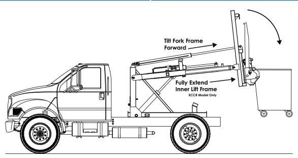
2. Tilt the fork frame forward and fully extend the inner lift frame(ECCR Model Only).
