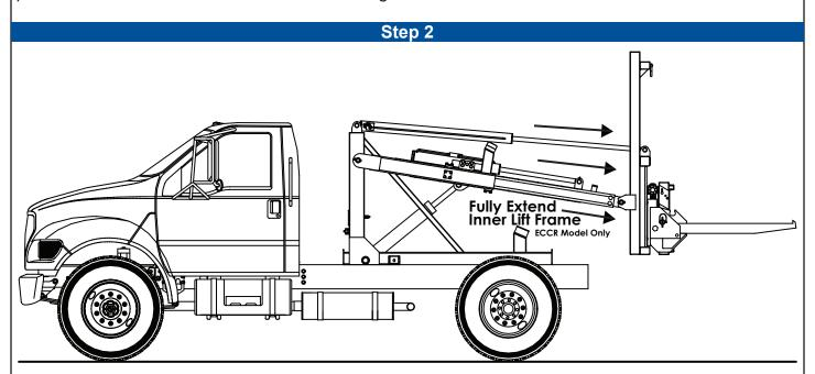
2. Fully extend the inner lift frame (ECCR Model Only).
