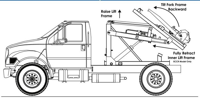
5. Raise the lift frame high enough to clear the truck frame. Fully retract the inner lift frame (ECCR Model Only). Tilt the fork frame all the way up so full contact is made with the rest pads.
