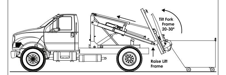
6. Raise the lift frame until the trunnion bars are securely located in the slots. Tilt the fork frame up approximately 20 to 30 degrees. Put both trunnion bar stops in the 'locked' position (See next page).
