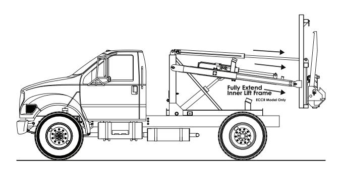
3. Fully extend the inner lift frame (ECCR Model Only).
