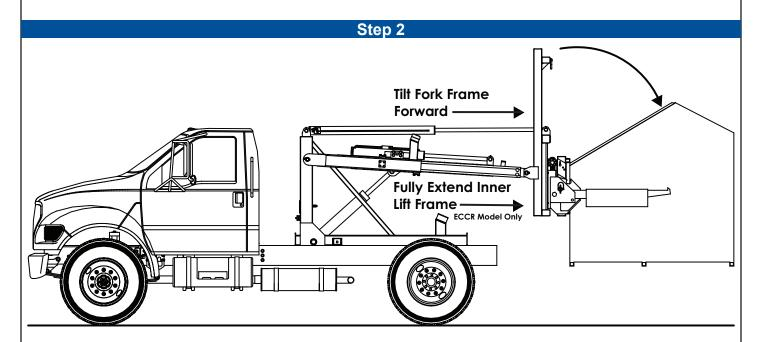
2. Tilt the fork frame forward until the container is parallel with the ground. Fully extend the inner lift frame(ECCR Model Only).
