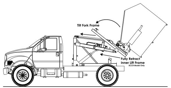
6. Fully retract the inner lift frame (ECCR Model Only). Tilt the fork frame all the way up so that full contact is made with the rest pads.
