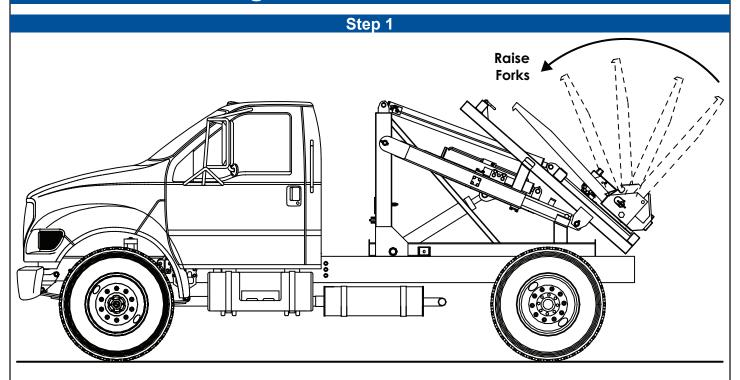
1. If the forks are in the extended position, manually rotate them to the stored position. Lock the forks in place with the fork stop pins.
