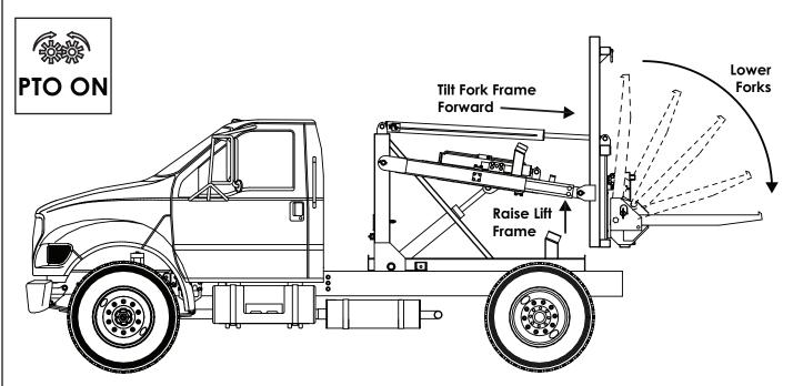
1. If the forks are in the stored position, engage the PTO and raise the lift frame high enough to clear the truck frame. Tilt the fork frame forward to allow easy manual rotation to the down position. Lock the forks into place with the fork stop pins.
