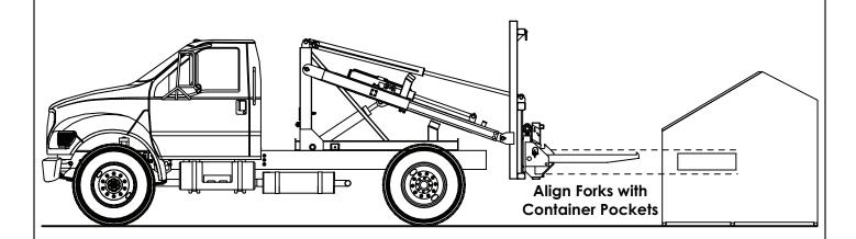
3. Align the forks with the container pockets by lowering the lift frame and tilting the fork frame.
