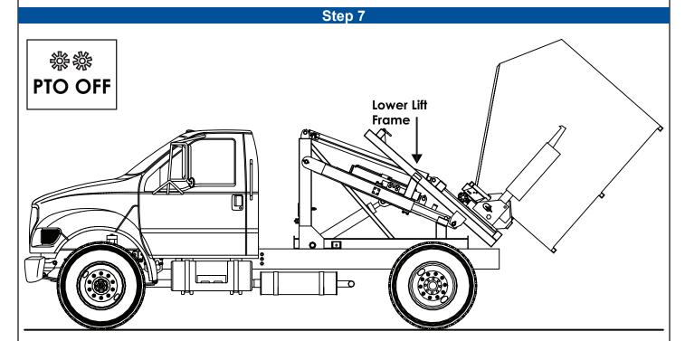
7. Lower the lift frame completely and disengage the PTO. Note: Check local DOT lighting regulations before transporting.
