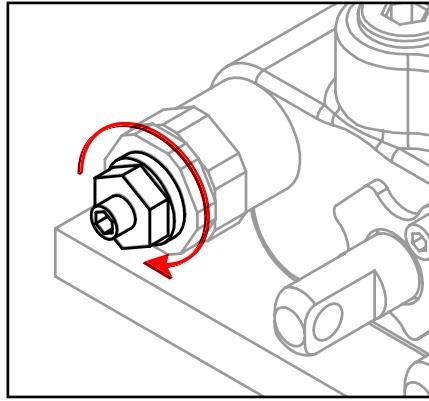
6. Release all functions and disengage the PTO. Snap tamper cap into position over the jam nut. The break away clip will be destroyed if the cap is removed.
