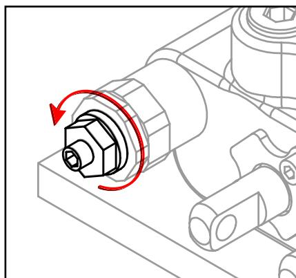
4. Adjust the system relief pressure using 4 mm allen wrench (See chart on previous page). Clockwise increases pressure, counter clockwise decreases pressure:
