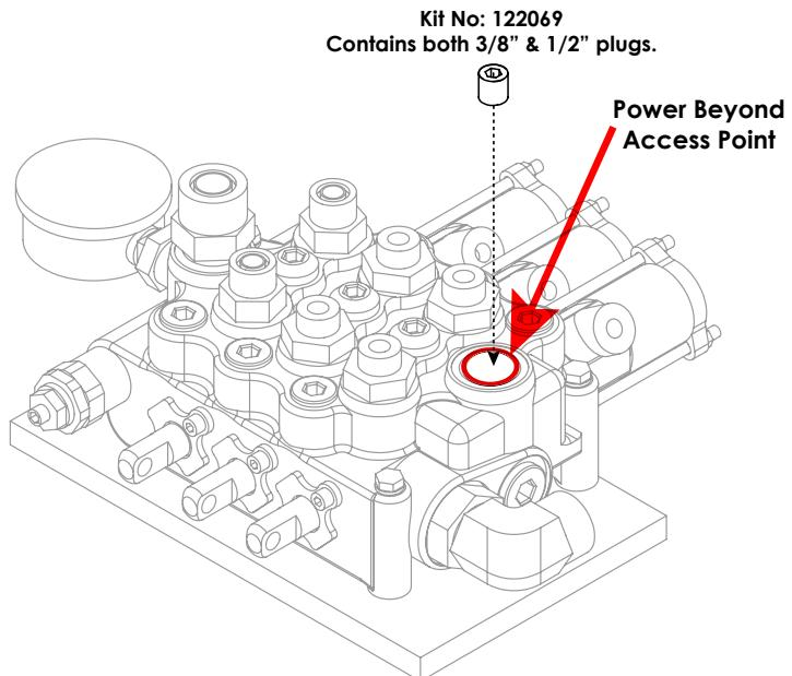
3. The Power Beyond feature is now activated and will divert oil to alternate system via the port shown.
