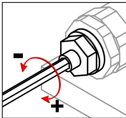
5. Once system pressure is set, tighten the jam nut to lock system pressure. Permanent thread lock should not be used:
