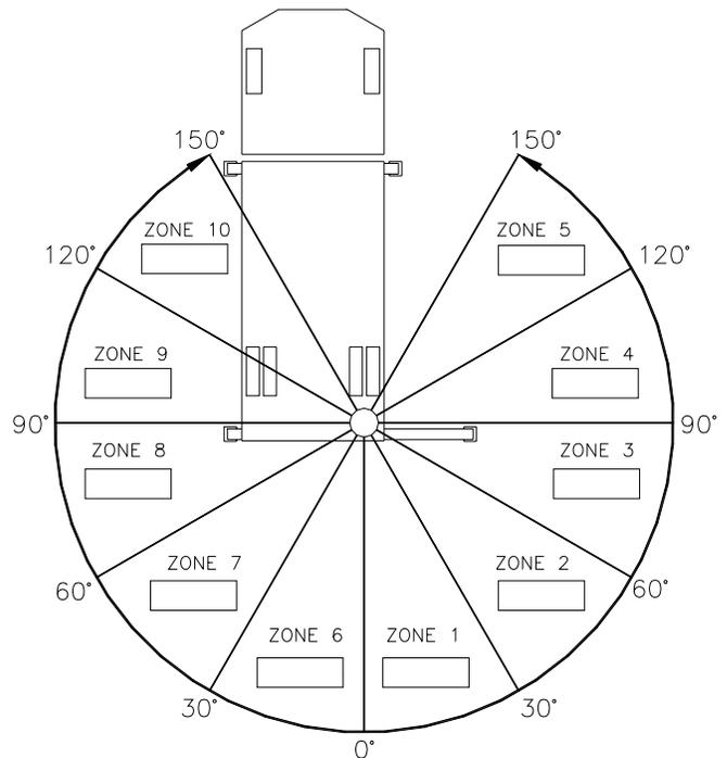
$$\frac{\text{Stable Horizontal Reach}}{\text{Max Horizontal Reach}} \times 100 = \text{Percentage of Rated Capacity}$$
