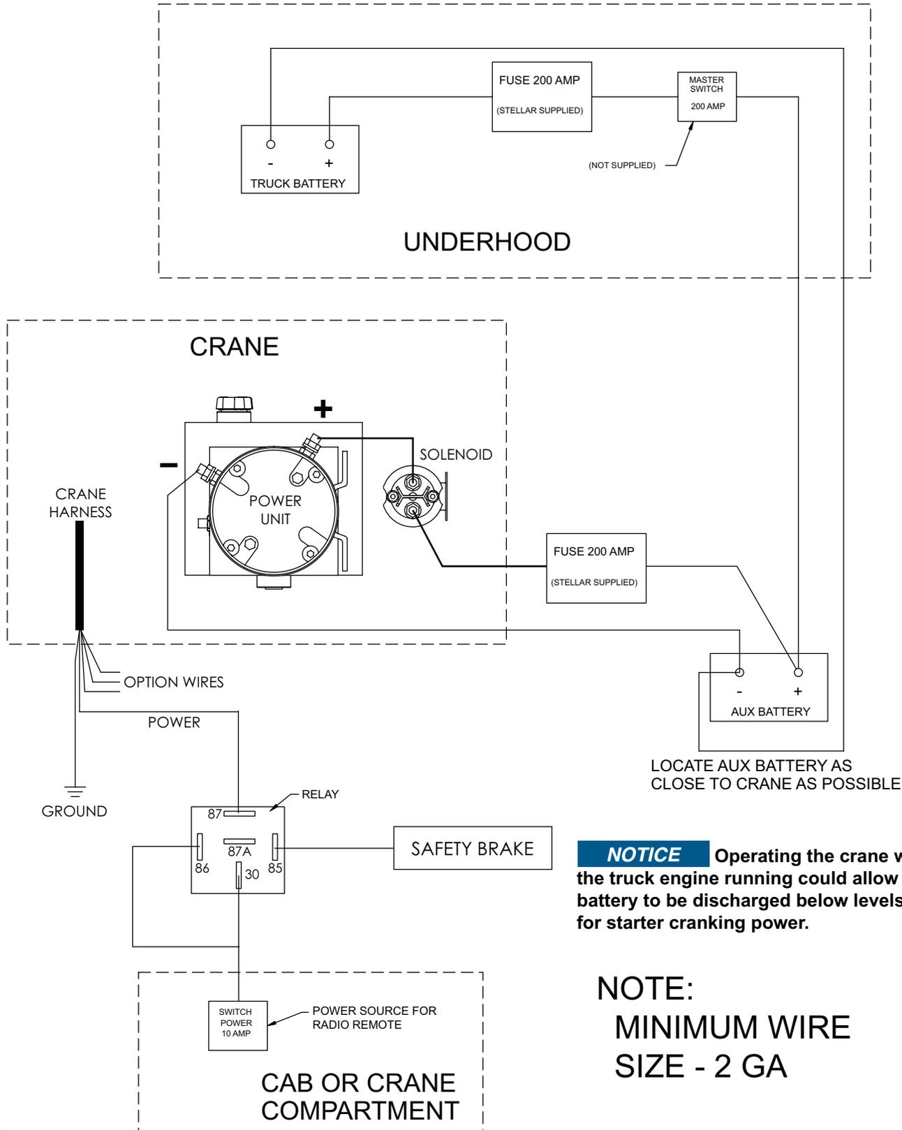
**NOTICE** Operating the crane without the truck engine running could allow the truck battery to be discharged below levels required for starter cranking power.
